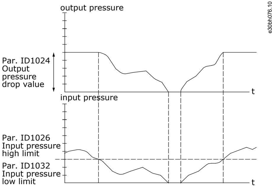
Illustration 87: Output Pressure Behavior Depending on Input Pressure and Parameter Settings
