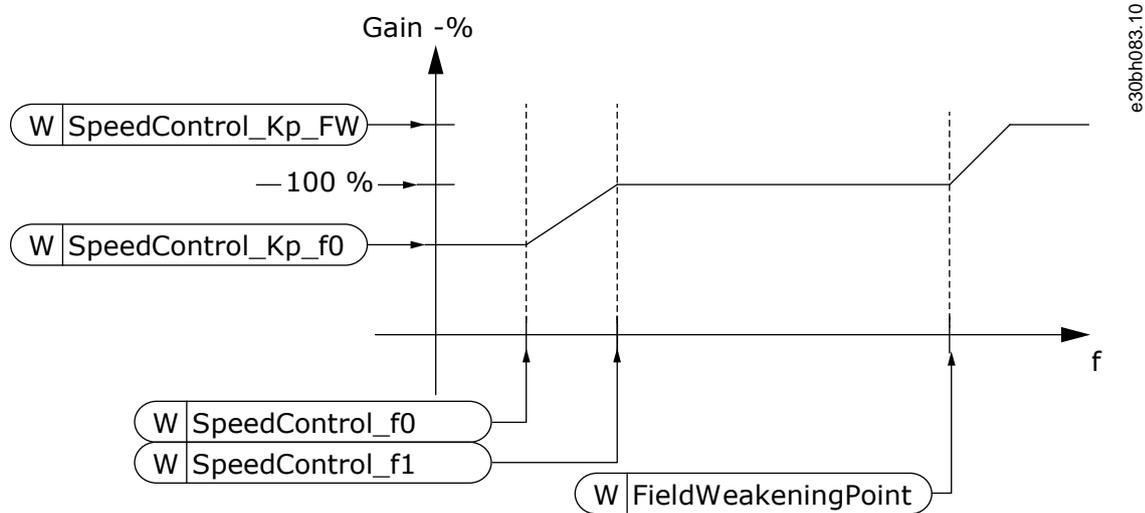
Illustration 101: Speed Controller Adaptive Gain
