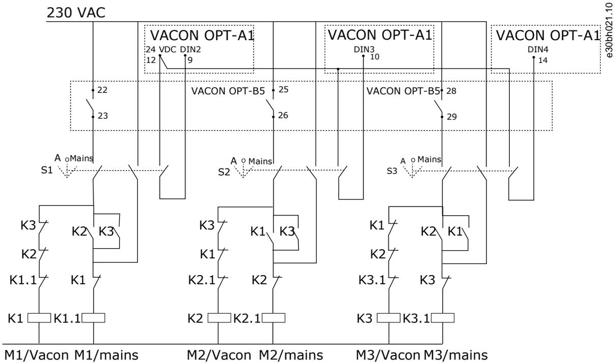
Illustration 23: Pump Autochange System, Principal Control Diagram
