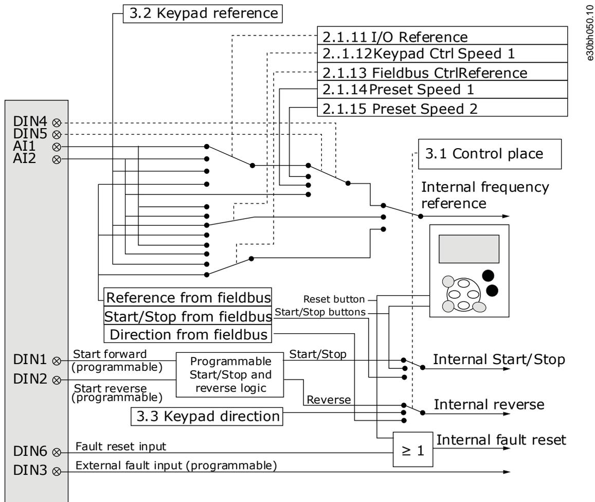
Illustration 7: Control Signal Logic of the Standard Application
