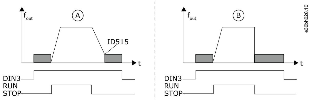
Illustration 34: DIN 3 as DC brake Command Input
