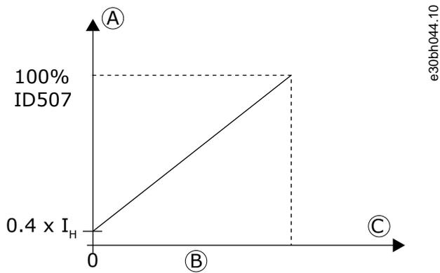
Illustration 52: Reduction of DC Braking Current
