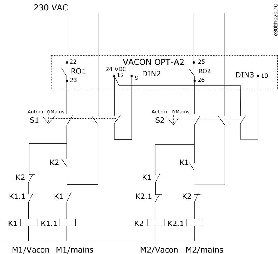
Illustration 22: Pump Autochange System, Principal Control Diagram
