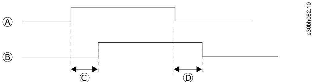
Illustration 66: Digital Outputs 1 and 2, On- and Off-Delays
