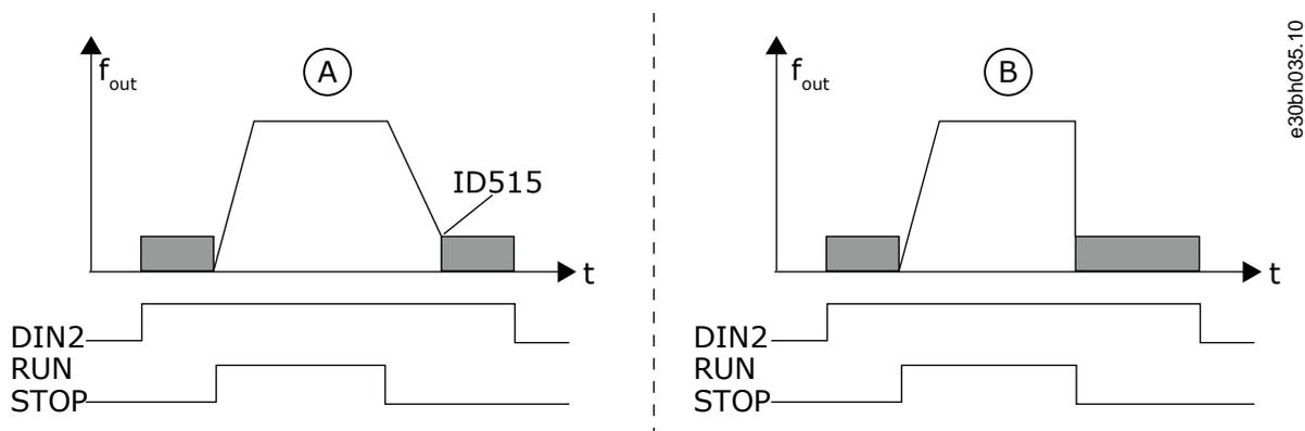
Illustration 42: DC Braking Command (Selection 12) Selected for DIN 2
