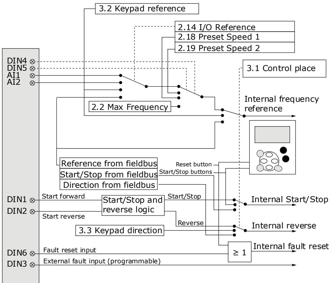
Illustration 4: Control Signal Logic of the Basic Application
