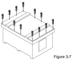
Unpacking 2 (VFDXXXCXXE, VFDXXXC63B-21) Loosen the 16 screws at the four corners of the crate, and then remove the iron plates.
