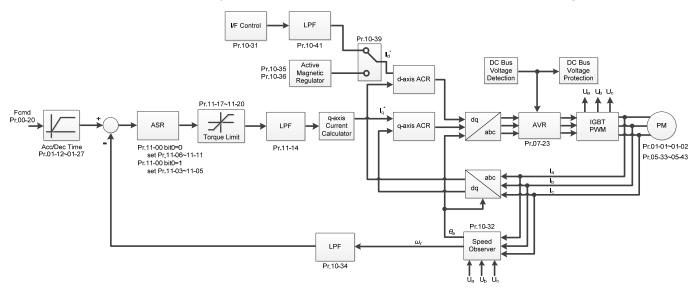
When Pr. 00-10=0, and you set Pr. 00-11 to 7, IPM FOC sensorless control diagram is as follows:
