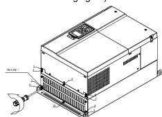
Fasten 5 screws (as shown in the following figure). Screw torque: 30~32 kg-cm / [26.0~27.8 lb-in.] / [2.9~3.1 Nm]
