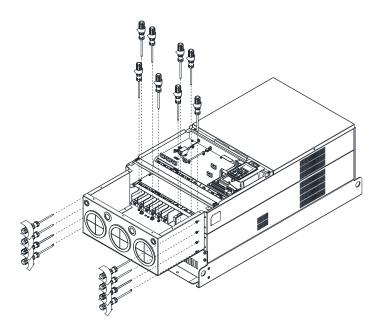
5. Fasten all the screws. Screw torque: 24~26 kg-cm / [20.8~22.6 lb-in.] / [2.4~2.5 Nm]
