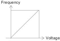
Fcmd=[(ay $\pm$ bias)\*gain]\*  $\frac{\text{Fmax}(01-00)}{10\text{V or }16\text{mA or }20\text{mA}}$
