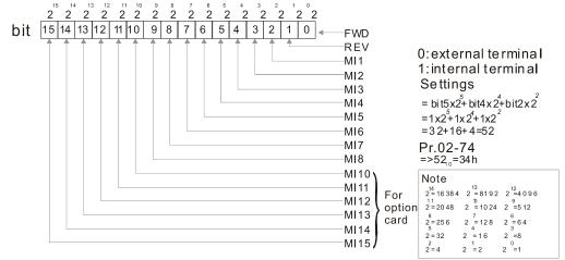
M G2-75 Internal Multi-function Output Terminal Selection
