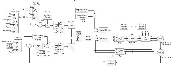
Pr. 00-13=2, IM TQC Sensorless control diagram is as follows:
