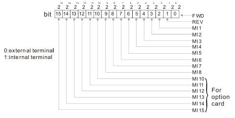
For example, if setting MI1, MI3 and MI4 to be ON, Pr.02-75 should be set to bit5X2<sup>5</sup>+bit4X2<sup>4</sup>+bit2X2<sup>2</sup>= 1X2<sup>5</sup>+1X2<sup>4</sup>+1X2<sup>2</sup>= 32+16+4=522 =34h as shown in the following.
