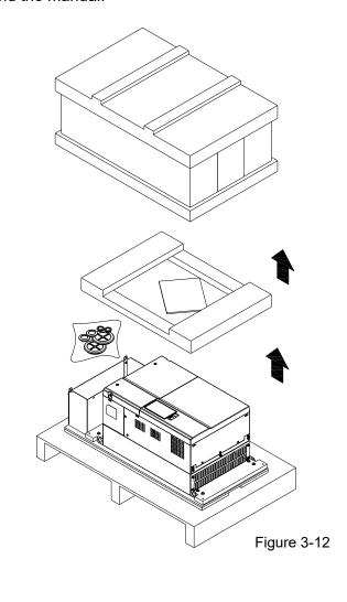
Loosen the eight screws fasten the drive on the pallet, and then remove the wood plate.
