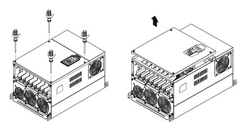
2. Fasten the 6 screws shown in the following figure and place the cover back to the original position. Screw torque: 24~26 kg-cm / [20.8~22.6 lb-in.] / [2.4~2.5 Nm]
