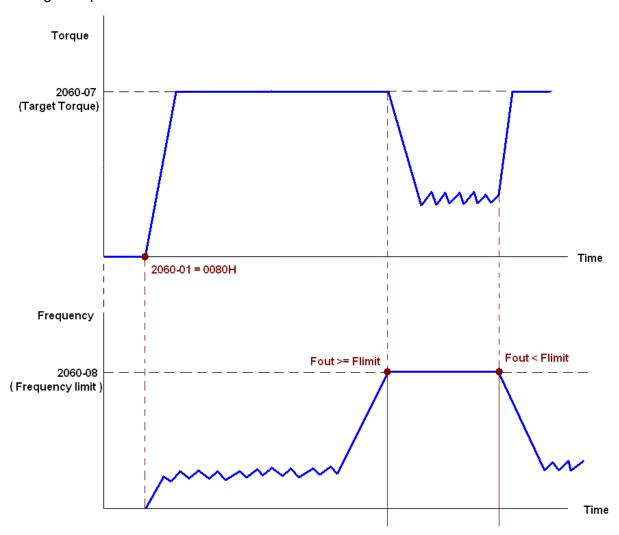
Note01: Read 2061-07 for the current torque (unit is 0.1%).
