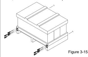
Unpacking 2 (VFDXXXCXXE, VFDXXXC63B-21) Loosen the 16 screws at the four corners of the
