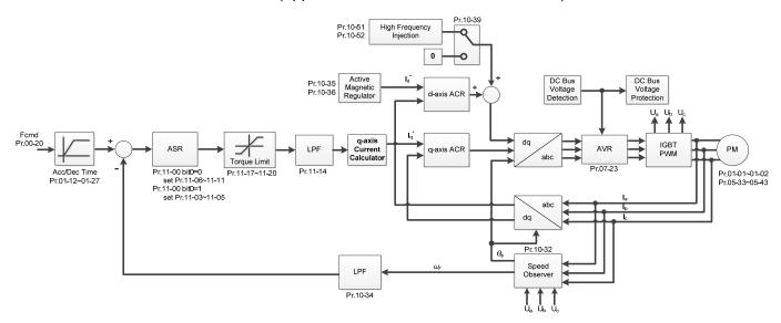
PM Sensorless FOC control is the control method dedicated for IPM, it uses the high salient pole characteristic (Lq > Ld) of IPM to detect the positions of NS magnetic poles. By doing this, it calculates the motor's rotor position at low-speed frequency.
