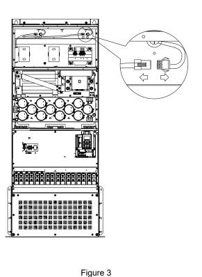
Loosen screws 1~4 (as shown below) and remove the fan. Make sure the fan is disconnected when removing. Screw torque: 24~26kg-cm / [20.8~22.6 lb-in.] / [2.4~2.5 Nm] (figure 4)
