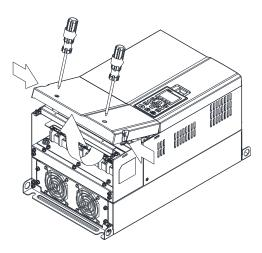
2. Remove the 5 screws shown in the following figure. Screw torque: 24~26 kg-cm / [20.8~22.6 lb-in.] / [2.4~2.5 Nm]
