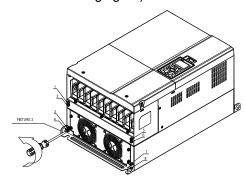
Fasten 4 screws (as shown in the following figure). 4. Screw torque: 30~32 kg-cm / [26.0~27.8 lb-in.] / [2.9~3.1 Nm].
