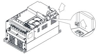
(Figure 2) Loosen screw 3, press the tab on the right and the left to remove the cover. Screw 3 Torque: 6~8 kg-cm / [5.2~6.9 lb-in.] / [0.6~0.8 Nm]
