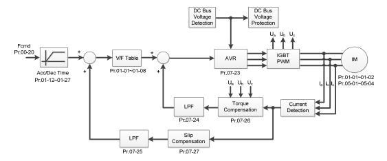
When Pr. 00-10=0, and you set Pr. 00-11 to 1, the V/F control + encoder diagram is as follows.
