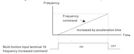
When Pr.02-09 is set to 1: the increasing / decreasing frequency command (F) operates according to the setting of Pr.02-10 (0.01–1.00 Hz/ms).
