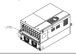
1. Loosen 8 screws and remove Fixture 2 (as shown in 2. Loosen 10 screws and remove Fixture 1 (as shown in the following figure).
