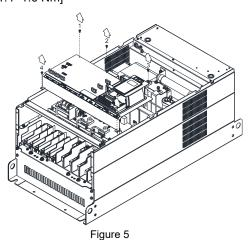
2. For 1~8 shown in the figure 2: Loosen the screws Screw torque: 35~40 kg-cm / [30.4~34.7 lb-in.] / [3.4~3.9 Nm]
