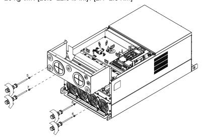
3. Install the conduit box by fasten all the screws shown in the following figure Screw 9~12 torque: 12~15 kg-cm / [10.4~13 lb-in.] / [1.2~1.5 Nm] Screw 13~16 torque: 24~26 kg-cm / [20.8~22.6 lb-in.] / [2.4~2.5 Nm]
