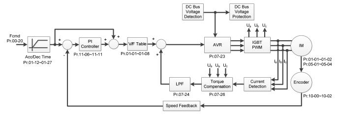
When Pr. 00-10=0, and you set Pr. 00-11 to 2, the space vector control diagram is as follows: IM Space Vector Control (IMSVC):
