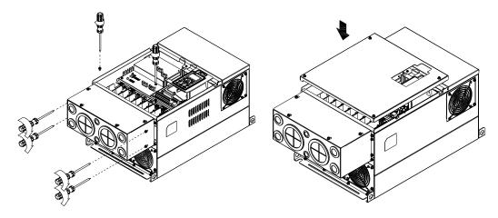
3. Fasten the 4 screws shown in the following figure. Screw torque: 12~15 kg-cm / [10.4~13 lb-in.] / [1.2~1.5 Nm]
