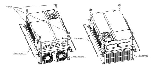
Plate installation, place 8 of the screw 2 (M6) through Accessory 1 & 2 and the plate then fasten the screws.
