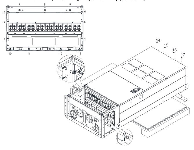
5. Fasten the 3 covers and screws, which were loosen from step 1, to the original location. Screw Torque:  $35\sim45$  kg-cm /  $[30.3\sim39$  lb-in.] /  $[3.4\sim4.4$  Nm]
