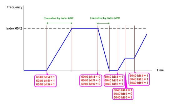
NOTE 01: Read 6043 to get the current rotation speed. (Unit: rpm)
