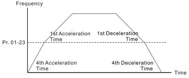
1st/4th Acceleration/Deceleration Frequency Switching
