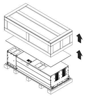
Loosen the six screws fasten the drive on the pallet, and then remove six metal washers and six plastic washers. See the figure below.
