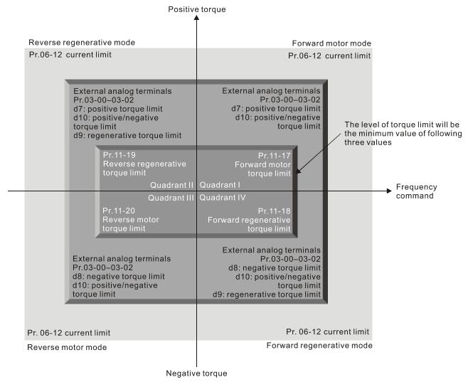
The control mode is based on 100% motor rated current except for these four modes: IM: VF, VFPG, SVC / PM: PMSVC modes.
