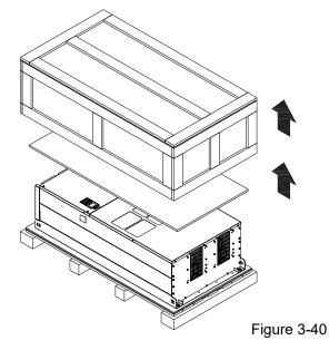
Remove the top cover, take out the EPEs, rubber and the manual.
