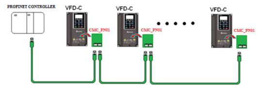
When the installation is finished, supply electricity to the drive. The Pr.09-60 of the drive should be able to display "PROFINET" with a current value of 12. If not, make sure your version of the drive is correct (C2000 needs 2.04 or later versions) and the communication card is correctly connected.
