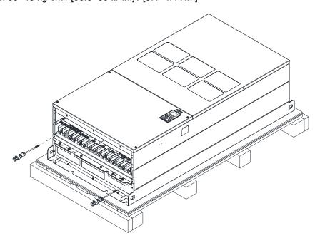
4. Install the conduit box by fasten all the screws shown in the following figure. Screw 1~6: M6 screw torque: 55~65 kg-cm / [47.7~56.4 lb-in] / [5.4~6.4 Nm] Screw 7~9: M8 screw torque: 100~110 kg-cm / [86.7~95.4 lb-in] / [9.8~10.8 Nm] Screw 10~13: M10 screw torque: 250~300 kg-cm / [216.9~260.3 lb-in] / [24.5~29.4 Nm] Screw 14~17: M8 screw torque: 100~110 kg-cm / [86.7~95.4 lb-in] / [9.8~10.8 Nm]
