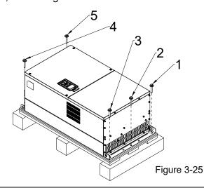
Loosen the five screws fasten the drive on the pallet, and then remove the wood plates.
