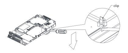
As shown in the figure on the left. Twist to open the clip. Insert a slot type screwdriver into the hollow to prize the PCB off the clip.
