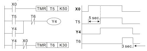
Example 12: Extended timing circuit
