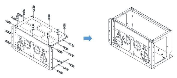
2. Loosen the screws as below figure shown.
