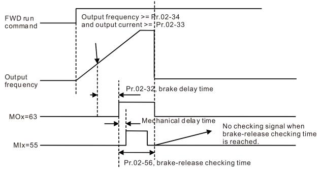
Multi-function output terminal: Function 42: Brake Current Check Point
