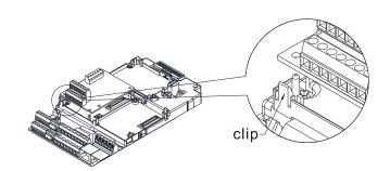
As shown in the figure on the left. Twist to open the other clip to remove the PCB.
