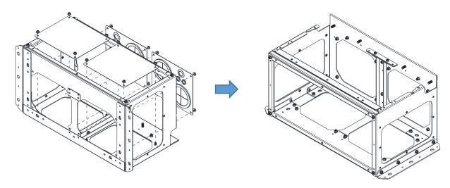
3. Remove the parts and screws as below figure shown.
