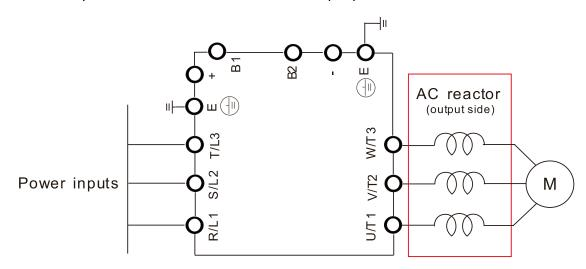
Wiring of AC output reactor
