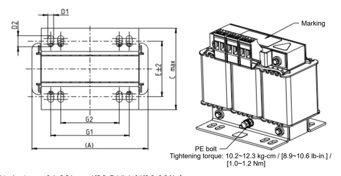
Tightening torque: 6.1~8.2 kg-cm / [5.3~7.1 lb-in.] / [0.6~0.8 Nm]
