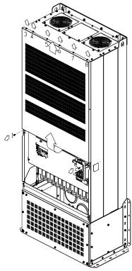
Loosen the screw 1~8 and remove the top cover (figure 2).
