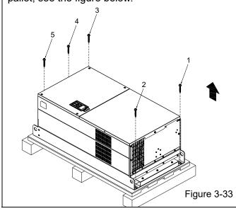
Loosen the 12 screws fasten the drive on the pallet, and then remove the wood plates.
