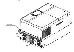
Place 4 screws (M10) through Fixture 1 & 2 and the plate then fasten the screws. (as shown in the following figure)
