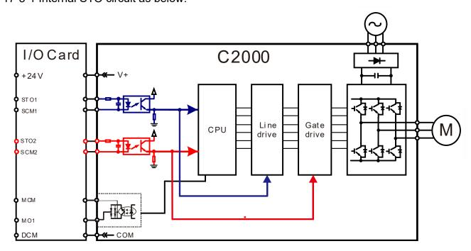
17-3-2 In the figure below, the factory setting for +24V-STO1-STO2 and SCM1-SCM2-DCM is short-circuited:
