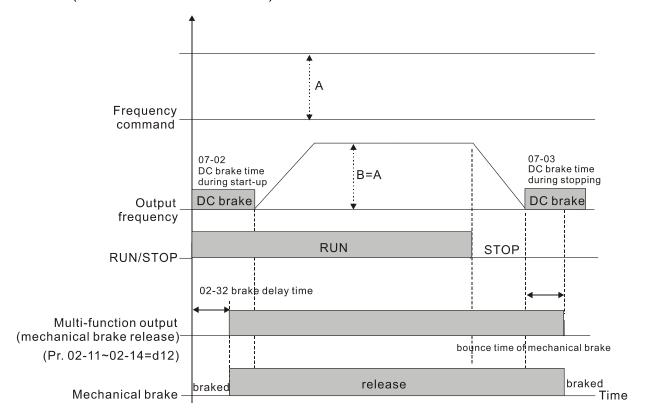
If this parameter is used without DC brake, it will be invalid. Refer to the following operation timing.
