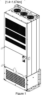
Loosen the screw 1~8 and remove the top cover (figure 2).
