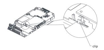
As shown in the figure on the left. Twist to open the other clip to remove the PCB.
