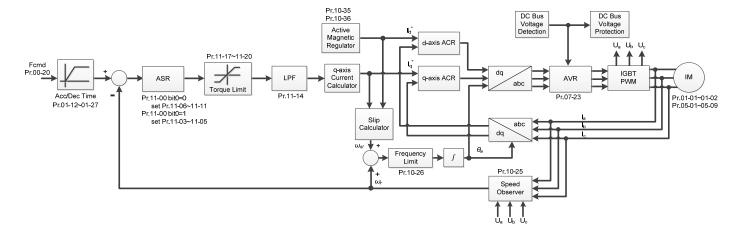
When Pr. 00-10=0, and you set Pr. 00-11 to 6, PM FOC Sensorless control diagram is as follows:
