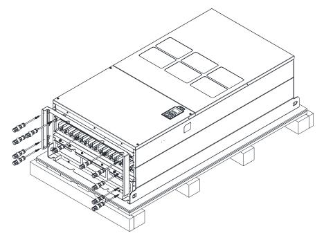
3. Fasten the M6 screws to locations shown in the following figure. Screw Torque: 35~45 kg-cm / [30.3~39 lb-in.] / [3.4~4.4 Nm]
