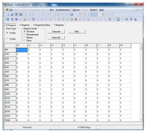
If there is a new PLC program and no settings have been made yet, you can read default data from the converter, and merely edit it to suit the current application.
