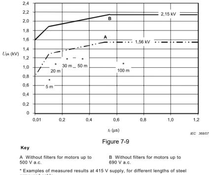
armoured cable Figure 14 – Limiting curves of impulse voltage  $U_{
