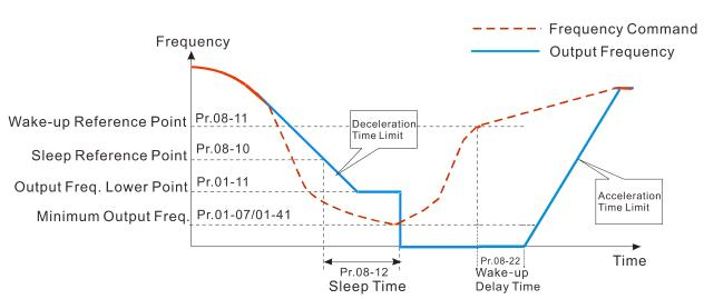
Internal PID Calculation Frequency Command
