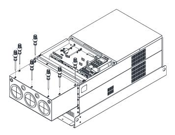
6. Place the cover back to the top and fasten the screws (as shown in the figure). Screw torque: 12~15 kg-cm / [10.4~13 lb-in.] / [1.2~1.5 Nm]
