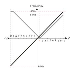
Pr.00-21=0 (Digital keypad control and run in FWD direction) Pr.03-05 Analog Positive Voltage Input Bias (AUI) = 10% Pr.03-07~03-09 (Positive/Negative Bias Mode)
