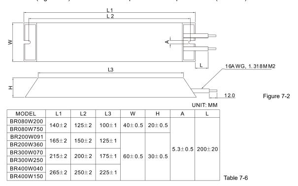
2. Select the resistance value, power and brake usage (ED %) according to Delta rules.
