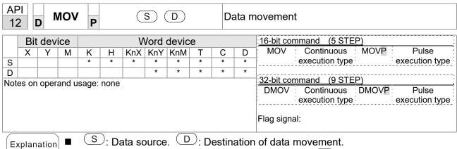
■ When this command is executed, the content of S will be directly moved to D. When the command is not executed, the content of D will not change.
