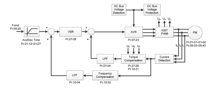
When Pr. 00-10=0, and you set Pr. 00-11 to 3, the IM FOCPG control diagram is as follows:
