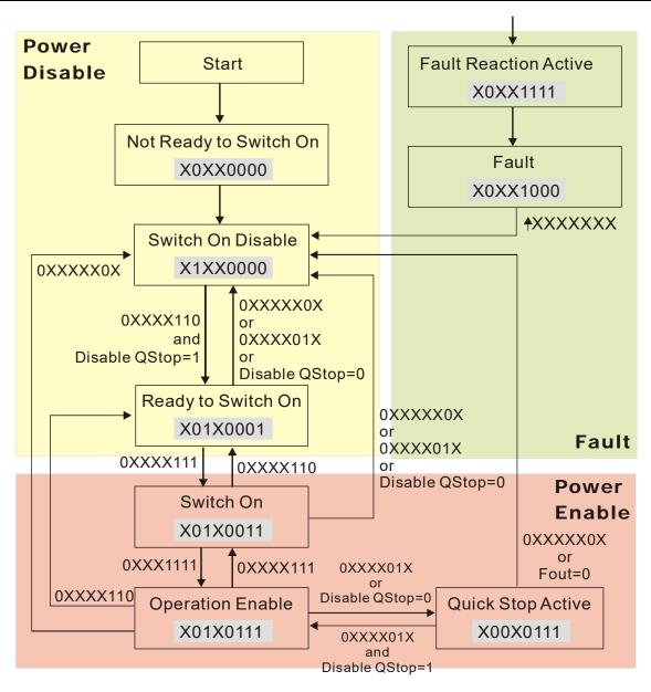
Set command 6040=0xE, then set another command 6040=0xF. Then you can switch the motor drive to Operation Enable. The Index 605A determines the lines from Operation Enable when the control mode changes from Quick Stop Active. When the setting value is 1–3, both lines are active, but when the setting value of 605A is not 1–3, once the motor drive is switched to Quick Stop Active, it is not able to switch back to Operation Enable.)
