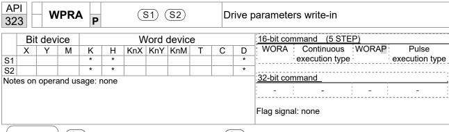
S1: Data that is going to write in S2: Parameter address of the write-in data
