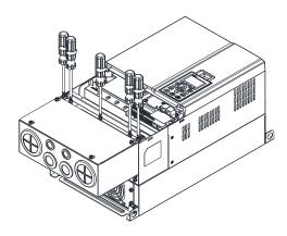
4. Fasten the 2 screws shown in the following figure. Screw torque: 12~15 kg-cm / [10.4~13 lb-in.] / [1.2~1.5 Nm]
