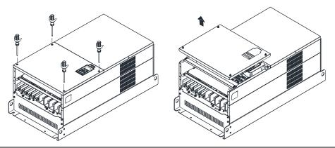
2. Remove the 5 screws from the FR4 board, as shown in the following figure. (The FR4 board is not needed after the installation of the power terminal kit). Screw Torque: 12~15 kg-cm / [10.4~13 lb-in] / [1.2~1.5 Nm]
