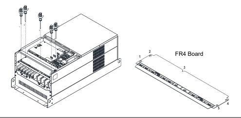
3. Loosen the upper M8 nuts (1~6) with a sleeve wrench (12mm of the sleeve). M8 Torque: 90kg / [78.1 lb-in] / [8.8 Nm]
