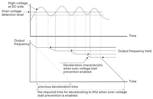
When you set Pr. 06-02 to 1, to use smart over-voltage stall prevention during deceleration, the drive maintains the DC BUS voltage when decelerating and prevents the drive from ov.
