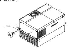
Fasten 5 screws (as shown in the following figure). Screw torque: 24~26 kg-cm / [20.8~22.6 lb-in.] / [2.4~2.5 Nm]
