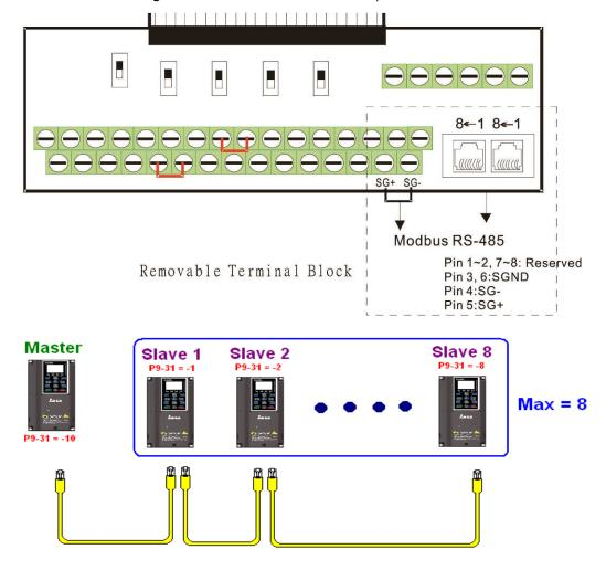
Master programming: In a program, D1110 can be used to define a slave station to be controlled (1–8, if set as 0, can jump between 8 stations). Afterwards, M1035 is set as 1, and the memory positions of the master and slave stations will correspond. At this time, it is only necessary to send commands to the correlation slave station address to control that station. The following is a register table connected with internal communications:
