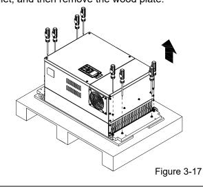
Loosen the ten screws fasten the drive on the pallet, and then remove the wood plates.
