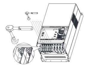
4. Install the 3pcs copper assy., as shown in the following figure 1. Fasten the upper M8 nuts (1~6) with a sleeve wrench (12mm of the sleeve), as shown in the figure 2 below.
