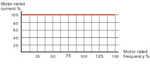
Motor cooling curve with shaft-fixed fan Motor cooling curve with independent fan
