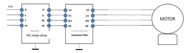
Wiring of non-shielded cable
