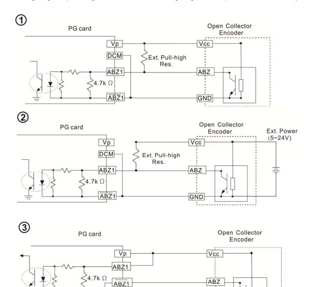
When wiring in this way, if there is a signal on EMC-PG010's A1, B1 and Z1, LED lights is OFF.
