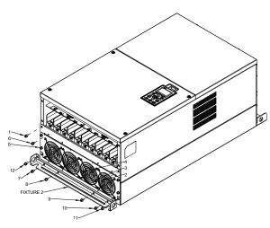
2. Loosen 12 screws and remove Fixture 2. Screw torque: 24~26 kg-cm / [20.8~22.6 lb-in.] / [2.4~2.5 Nm]
