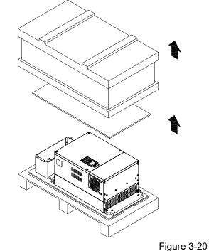
Loosen the eight screws fasten the drive on the pallet, and then remove the wood plate.
