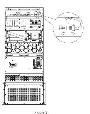
4. Loosen screws 1~6 (as shown below) and remove the fan. Make sure the fan is disconnected when removing. Screw torque: 24~26kg-cm / [20.8~22.6 lb-in.] / [2.4~2.5 Nm] (figure 4)
