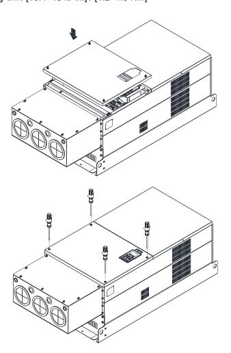
Assembly for Frame H3 (Conduit Box)
