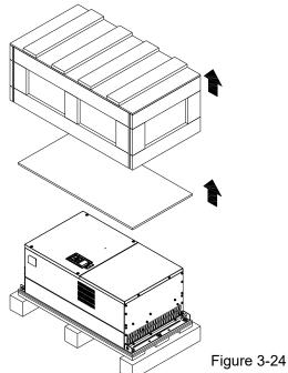
Remove the top cover, take out the EPEs, rubber and the manual.
