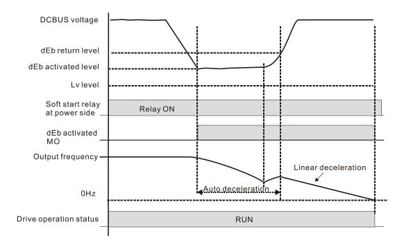
Situation 2: Momentary power loss, or power current too low and unstable, or power supply sliding down because of sudden heavy load.
