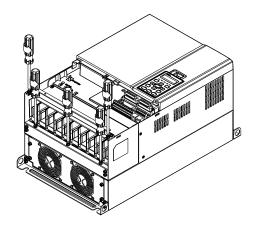
3. Install the conduit box by fasten the 5 screws shown in the following figure. Screw torque: 24~26 kg-cm / [20.8~22.6 lb-in.] / [2.4~2.5 Nm]
