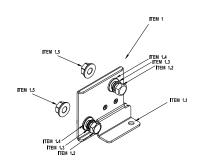
Diagram of power terminal connection M12 Torque: 408 kg-cm / [354.1 lb-in] / [39.98 Nm]
