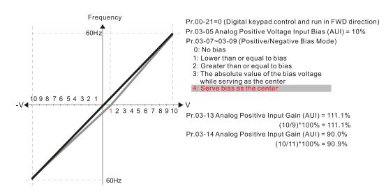
Reverse Setting when Analog Signal Input is Negative Frequency
