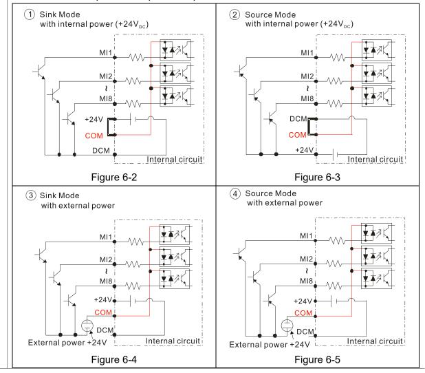
☑ When the photo-coupler is using internal power supply, the switch connection for Sink and Source as below:
