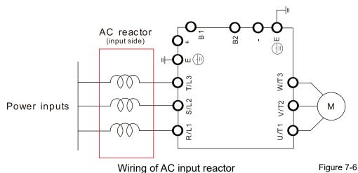
Following table shows the standard AC reactors specification of Delta C2000 200V~230V/ 50~60Hz
