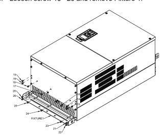
Install Fixture 1 by fasten screw 13 ~26
