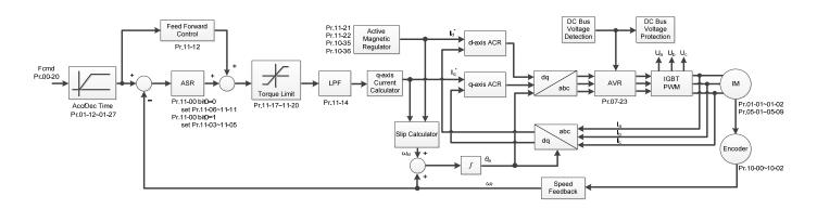
When Pr. 00-10=0, and you set Pr. 00-11 to 4, the PM FOCPG control diagram is as follows:
