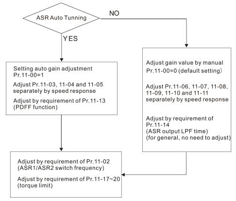
When the drive needs to keep a certain torque at zero-speed, or it needs a steady frequency output at extreme low speed, increase Pr. 11-05 zero-speed bandwidth appropriately. When the speed is in high-speed area, if the output current trembles seriously and makes the drive vibrate, then decrease the high-speed bandwidth.
