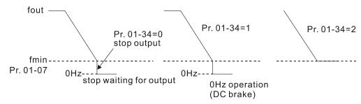
In FOCPG mode, when Pr. 01-34 is set to 2, the AC motor drive operates according to the setting.
