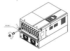
Fasten 4 screws (as shown in the following figure). 6. Screw torque: 24~26 kg-cm / [20.8~22.6 lb-in.] / [2.4~2.5 Nm]
