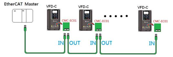
When the hardware is installed and power on, check for the display. The current set value of Pr.09-60 will be 6, and shows "EtherCAT" on the display. If the above information does not show on the display, please check the version of VFD-C2000 (V2.02 and above) and the connection of the card.
