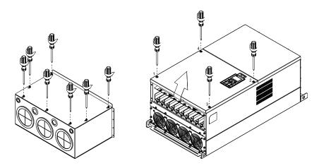
3. Remove the top cover and loosen the screws.
