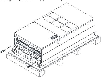
5. Install conduit box and accessories by fasten all the screws shown in the following figure.
