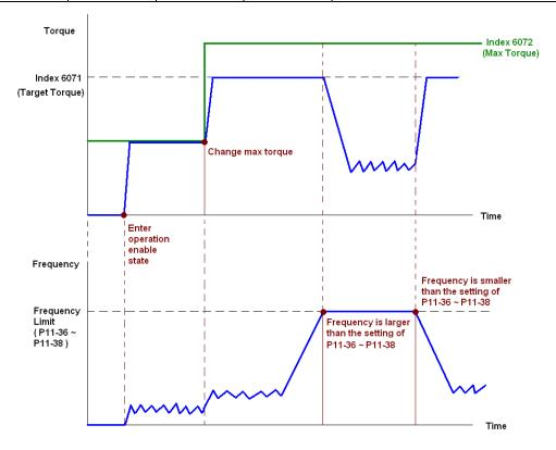
NOTE: The standard DS402 does not regulate the maximum speed limit. Therefore, if the motor drive defines the control mode of DS402, the highest speed will go with the setting of Pr. 11-36 to Pr. 11-38.
