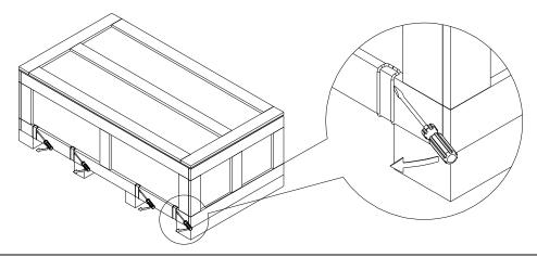
Remove the top cover, take out the EPEs, rubber and the manual.
